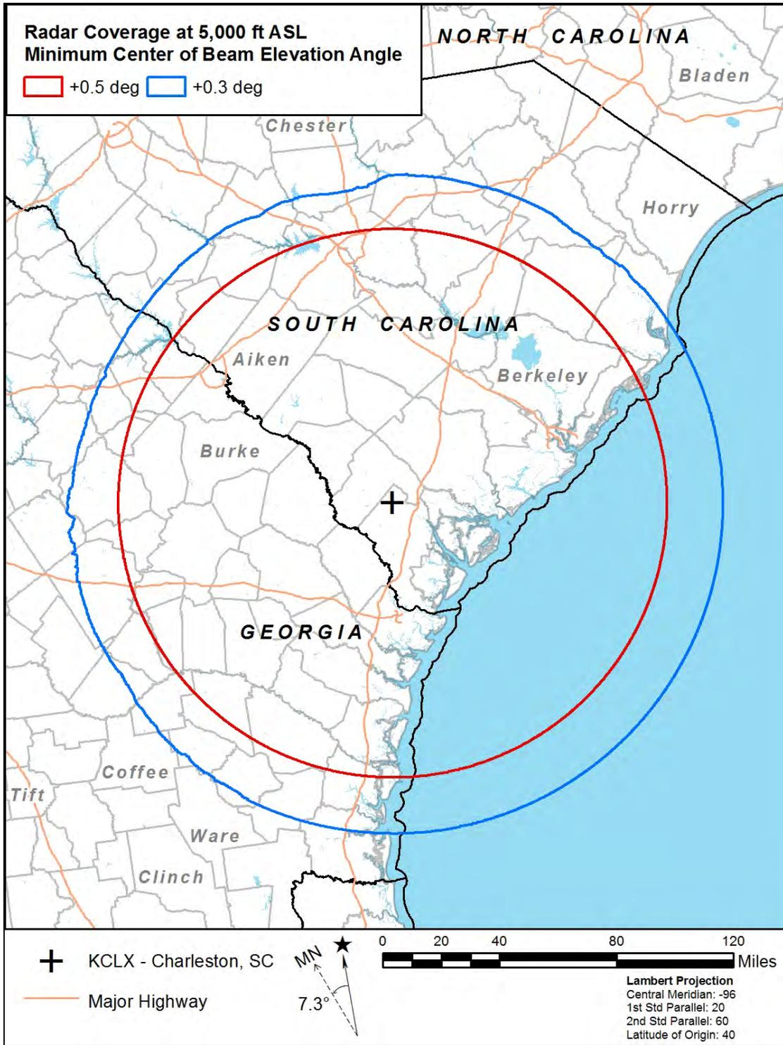
Figure 6: Existing and Proposed KCLX WSR-88D Coverage at 5,000 ft above Site Level
