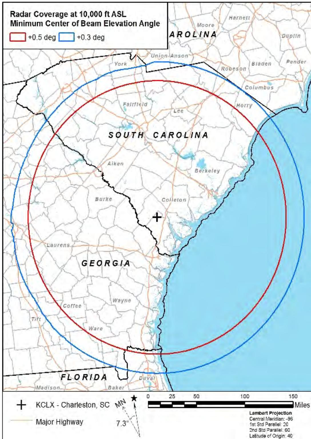
Figure 7: Existing and Proposed KCLX WSR-88D Coverage at 10,000 ft above Site Level
