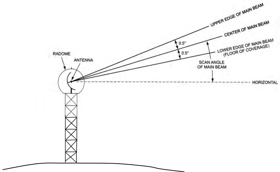
**Figure 3: Schematic of WSR-88D Main Beam**
