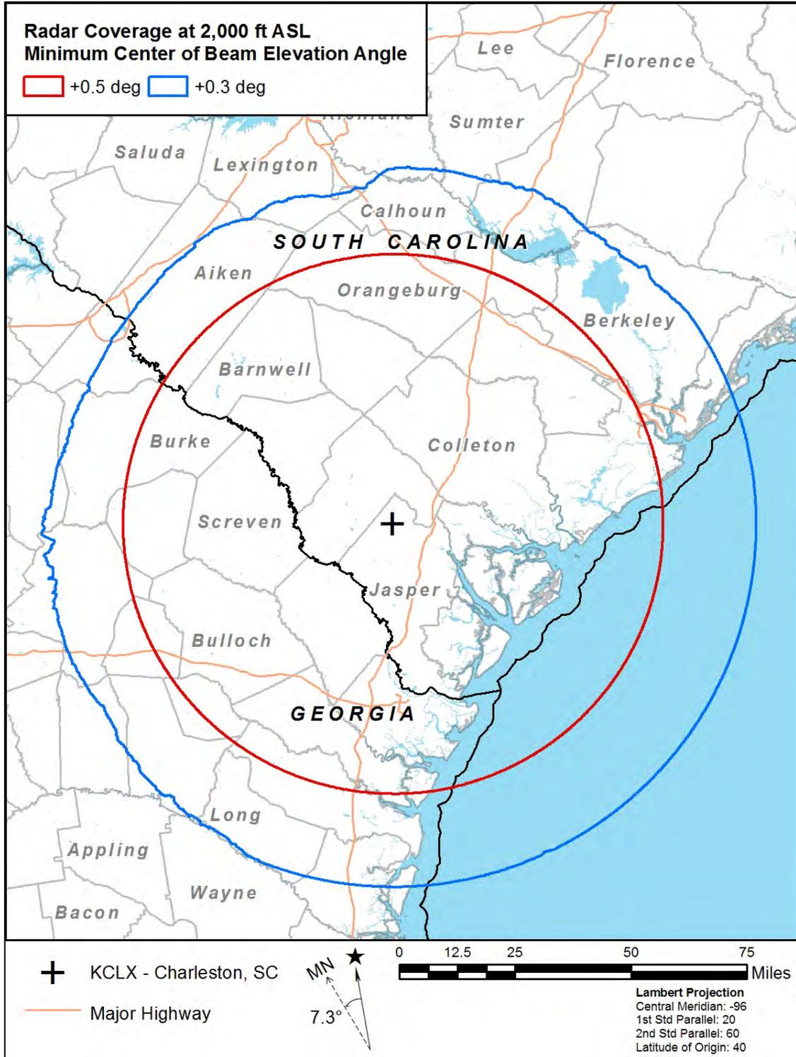
Figure 5: Existing and Proposed KCLX WSR-88D Coverage at 2,000 ft above Site Level
