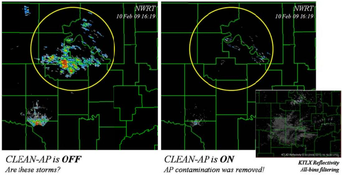
Figure 6 – CLEAN-AP Automatically Removing AP Clutter
