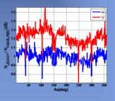
Legacy to radial measured noise ratio in the horizontal (H), and the vertical (V) channel.
