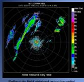
Reflectivity field obtained using the radial based noise measurement with additional detections highlighted in white.
