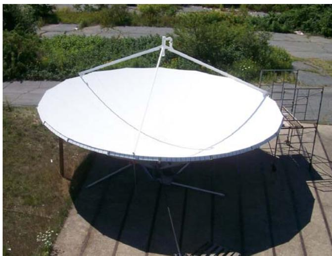
Figure 1. The WSR-88D Antenna
