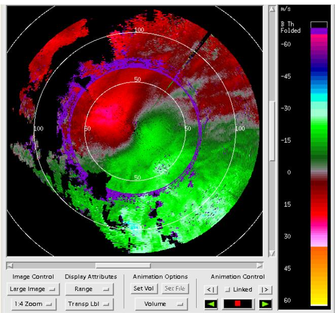
Figure 1c KCRI velocity image for same date and time as in Figure 1b. The 2<sup>nd</sup> and 3<sup>rd</sup> Doppler cuts were omitted thus simulating VCP 211. Note the band of range folding between 117 and 137 km. Range rings are same as Figure 1a.
