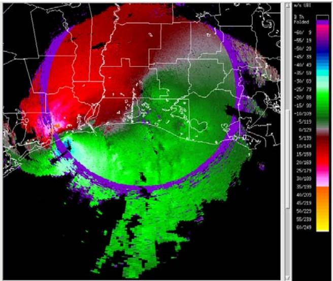
Figure 2c. KLCH Velocity image for same date and time as in Figure 2b. The 2<sup>nd</sup> and 3<sup>rd</sup> Doppler cuts were omitted thus simulating SZ-2 alone. Note the band of range folding between 117 km and 137 km that obstructs the peak winds in the eye (left center).
