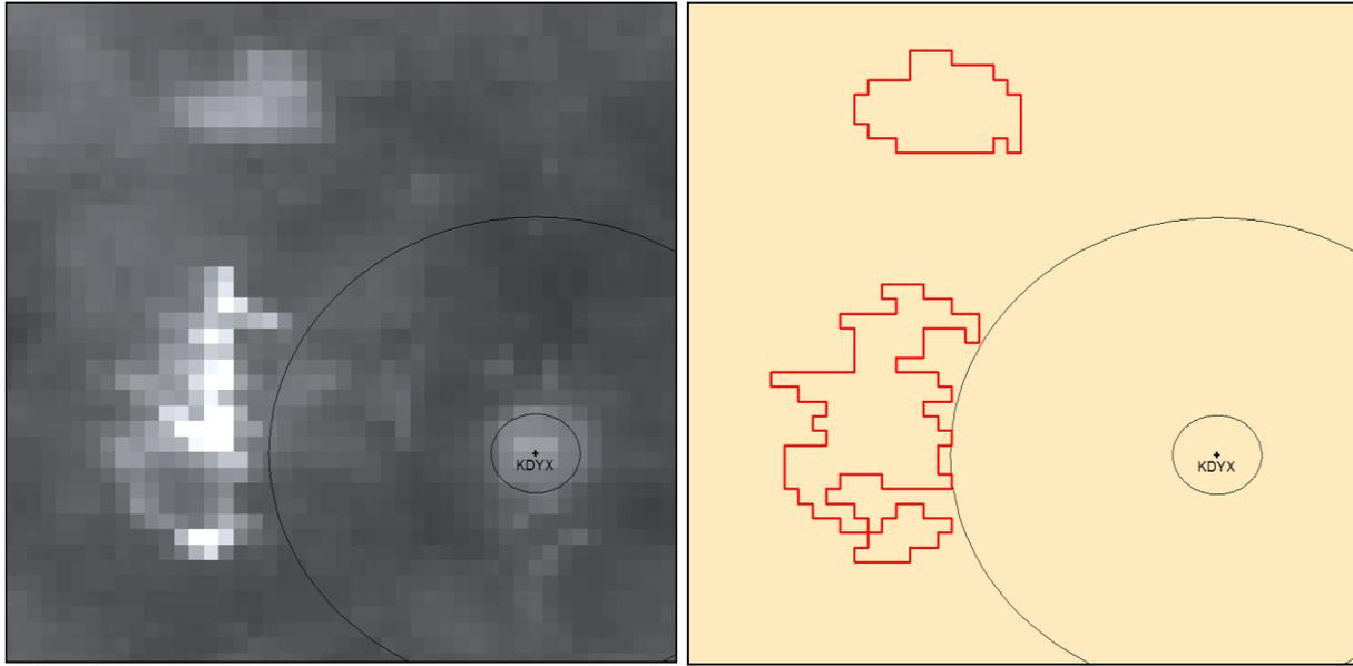
**Fig. 7.** Left image: 12-month Q2 QPE showing bright “hot spots” west of Dyess AFB WSR-88D (KDYX) near Abilene, TX with 3- and 18-km range rings. Right image: NSSL-generated polygons outlining QPE “hot spots”.
