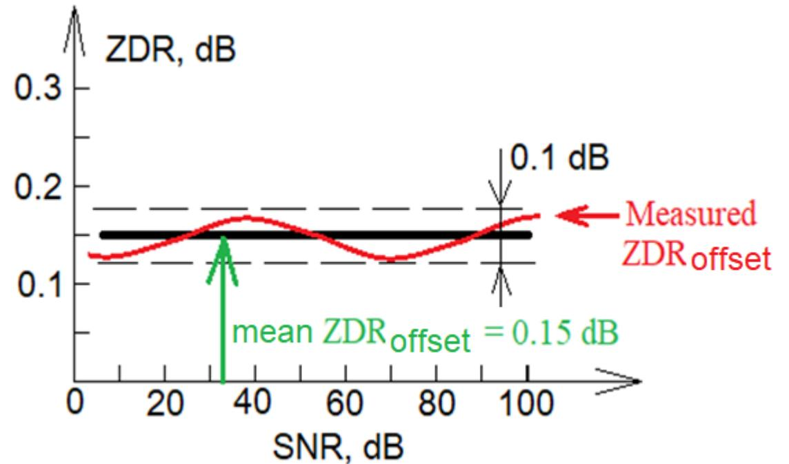
To measure ZDR with an accuracy of 0.2 dB, a radar receiver should be linear to 0.1 dB
